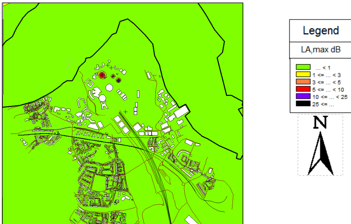
Figure 15.3.9 Calculated daytime levels L_{A,max,f} dB(A) for the area surrounding The Kent Project Site, with the Gate 1 and Gate 2 rides and attractions in operation (and baseline road traffic noise considered).
