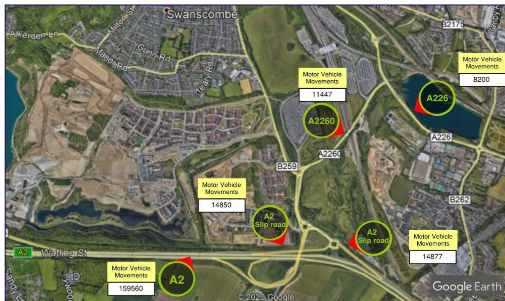
Figure 15.1.3. 2018 average daily flow of motor vehicles (Source: Department of Transport, Road traffic statistics).
